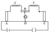
17. The figure above shows experimental set up of a meter bridge. Mention and state the principle of a meter bridge. When the two unknown resistances X and Y are inserted, the null point D is obtained 40 cm from the end A. When a resistance of 10  $\Omega$  is connected in series with X, the null point shifts by 10 cm. Find the position of the null point when the 10  $\Omega$  resistance is instead connected in series with resistance 'Y'. Determine the values of the resistances X and Y.
